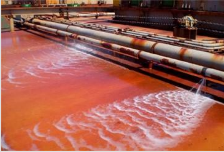
Holes in the fire main of the ship are causing water to leak out
